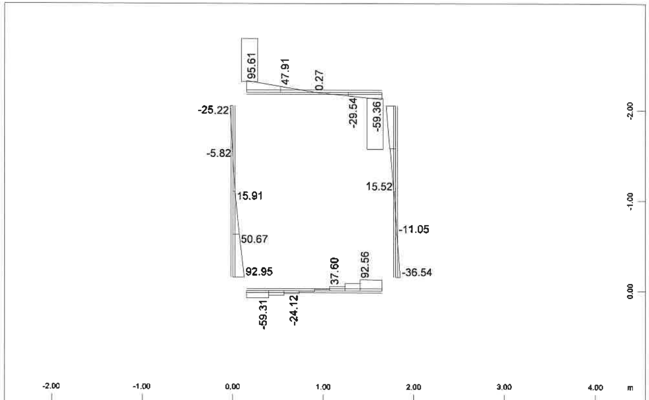
Sector of system Beam Elements Beam Elements , Shear force Vz, Loadcase 703 MAX-VZ BEAM , 1 cm 3D = 300.0 kN (Min=-59.4) (Max=95.6)
